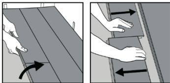
Separate the whole row by lifting it up delicately at an angle. To separate the planks, leave them flat on the ground and slide them apart. If planks do not separate easy, you can slightly lift up the planks (5°) when sliding them apart.
